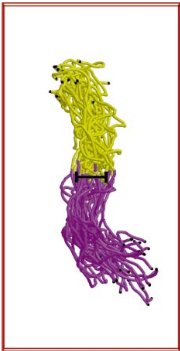
Figure 19. Visualization of the time evolution of a single primitive path constructed from block copolymer of N = 400 and \tilde{\epsilon} = 9.0 with N_c = 35 . The system is in the strongly segregated regime. The tube diameter d_T \approx 5\sigma , as found in the homopolymer melts, is indicated by the black bar. The total time of the run is 200000\tau with an increment of 6500\tau between the different conformations shown. The cell which is plotted here is only a fraction of the full simulation cell. The dimensions of the cell here and in the next figure are L_\perp = 60.0\sigma and L_\parallel = 30.0\sigma .
